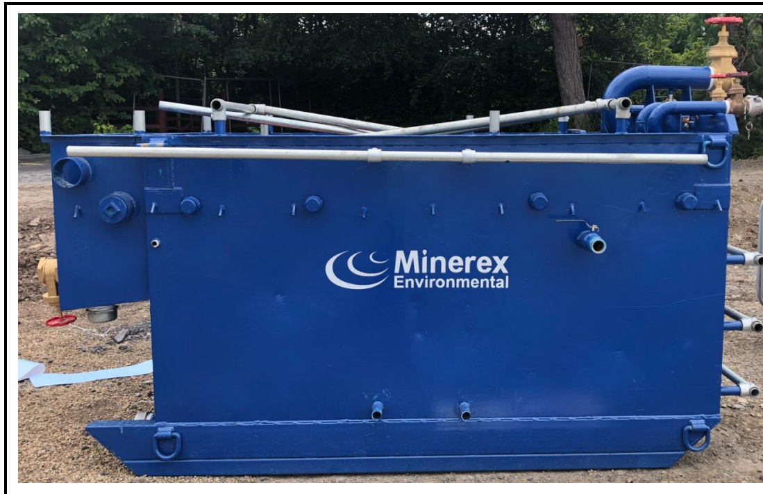
Example of an oil-water separator Minerex Environmental Limited, an RSK Group company
